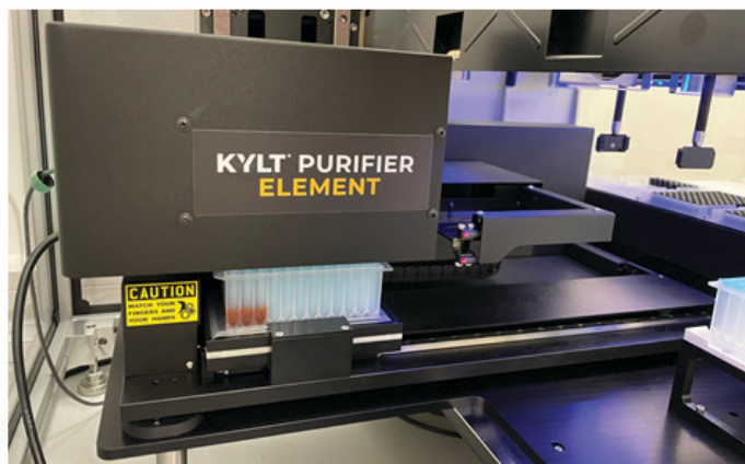
Figure 4: The KYLT Purifier Element device integrated on the Hamilton STARlet platform. Detailed view of the integration space.
